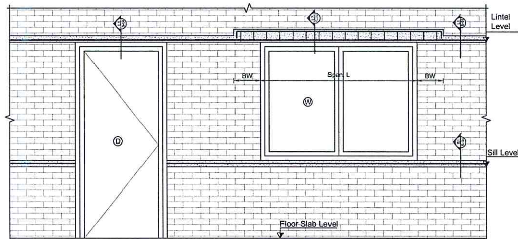
TYPICAL SILL AND LINTEL PROFILE DETAILS SCALE=1:30
